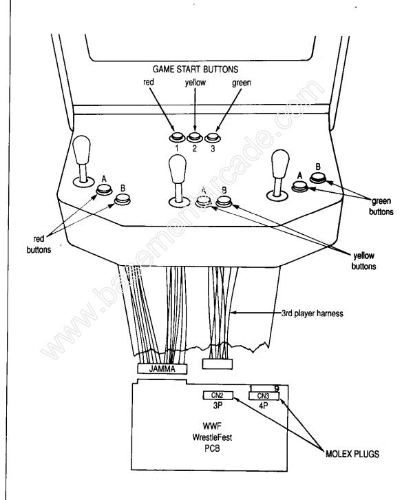
When making this 3-player conversion, you must use the 3rd player harness that has been supplied. Refer to earlier Diagram (A) on page 10 for connecting information. Make certain that dip switch bank number 2 has switch #3 ON and #4 OFF.
